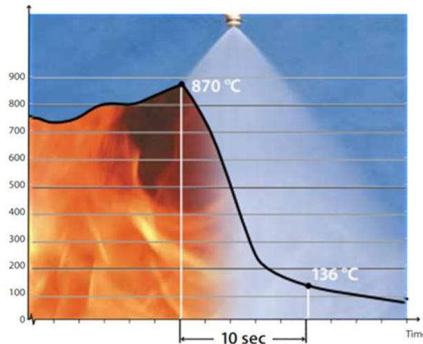
*In this simulation the fire is allowed to burn for more than 20 seconds. The burnt gas temperature increases to 870 °C at which point the FOGMAKER system is activated manually. In 10 seconds the temperature of the burnt gases decreases to approximately 136 °C. In addition to the rapid extinguishing the risk of re-ignition is minimized. This means reduced repairs and downtime.*
