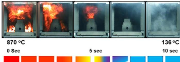
*Fire suppression test in a simulated engine compartment with a volume of 2.5 m<sup>3</sup>. The fire source consists of 4 20cm x 40cm trays filled with diesel. A spray fire is then simulated by applying diesel at a rate of 2 litres per minute at a pressure of 5 bar, which engulfs the engine. The combined heat output of the fire is approximately 1600 kW.*
