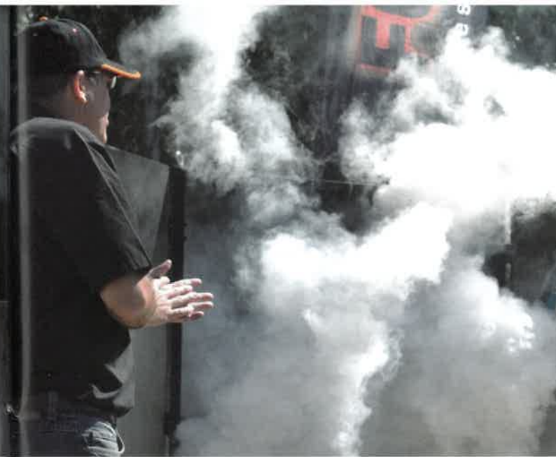
The Fogmaker high pressure water mist system suppressed the simulated fire within 10 seconds and reduced the temperature to below 100 degrees C
