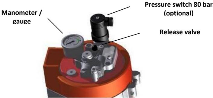
On delivery the extinguisher cylinder is filled to approx 105 bar pressure. The propellant consists of nitrogen gas. The pressure can be read off on a manometer and shall be within the green sector. The extinguisher cylinder is also available in a version with two or three connected cylinders. It can be located in a red protection box. As an option there is a pressure switch that gives an alarm if the pressure falls below approx 80 bar.
