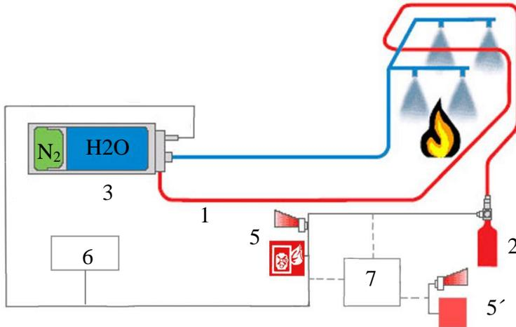
In the event of fire the detector hose bursts. When the pressure drop in the detection system has fallen to approx 10 bar a valve on the extinguisher cylinder is activated and the system is released. The pressure switch on the detector cylinder sends an alarm to the driver position.
